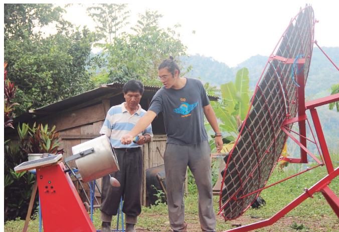
The roaster was designed to be used directly by coffee growers in field conditions, meaning it was easy to use and maintain, resistant, transportable and 100% solar operated.
